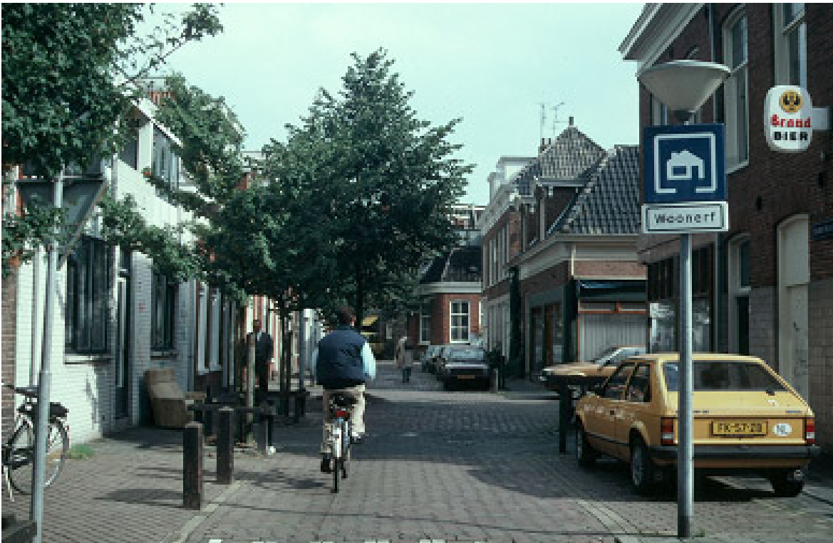
Woonerf design - a Dutch term meaning Living Street - shared with bicyclists, pedestrians and slow moving motor vehicles
