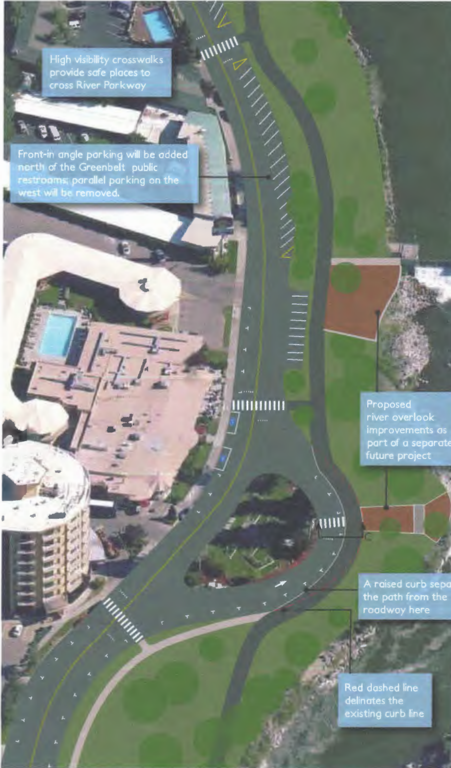
This section highlights changes to the existing bus and truck turnaround area, including removed parking from the inside of the bulb, adding a crossing between the island and a proposed river overlook, and adding front-in angle parking.
