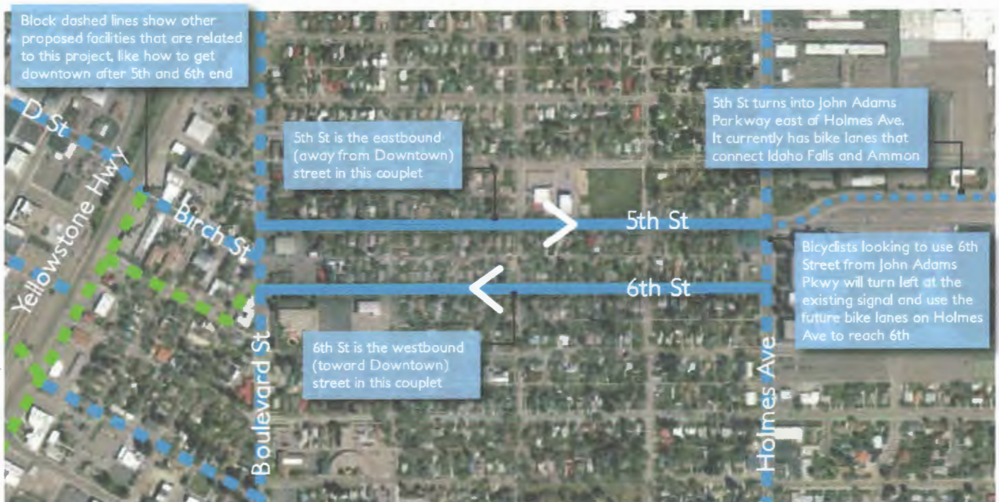
This aerial map shows the proposed bike lane or shared lane marking couplet project, how it connects to existing bike lanes and how it provides a key connection to Downtown Idaho Falls.
