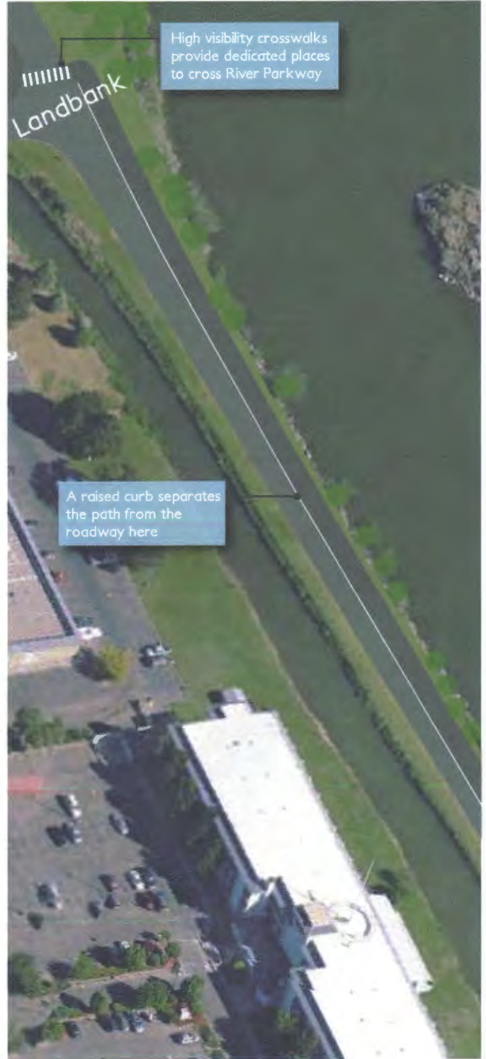
This section of River Pkwy is entirely one-way (northbound). Existing canal crossings allow hotel and restaurant patrons to access the Greenbelt Trail. Crossing improvements make these connections safer and more accessible. The existing 6' trail is widened to 14'. Landbank Street is seen in the top left of the figure at right.
