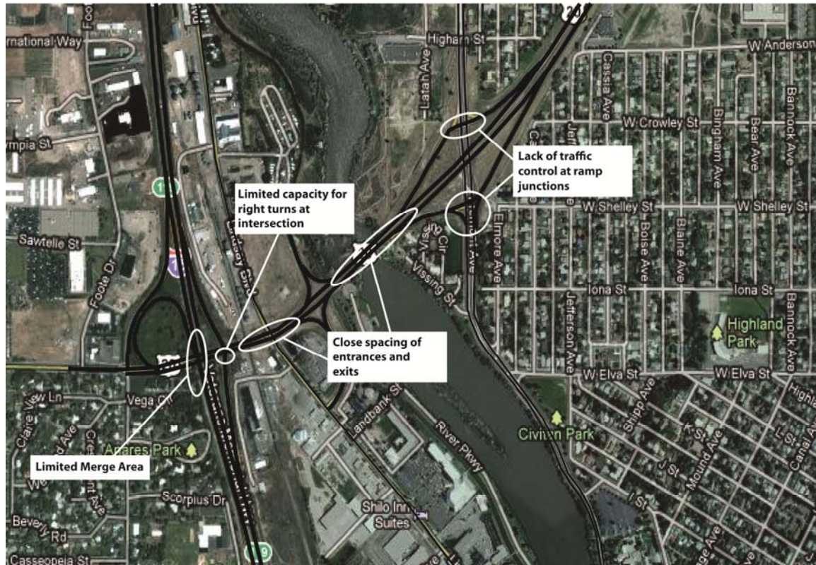
Figure 6-10 Capacity Issues in the I-15/US-20 Interchange Corridor
