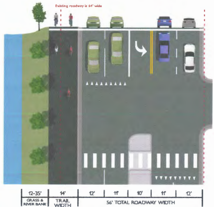
The intersection design for the preferred option of Riverside Dr and Snake River Greenbelt ( Project #2 ). Two travel lanes in each direction, a center turn lane, and median refuge (only at Elva St and the Temple), and a vegetated buffer instead of a center turn lane in all other locations.
